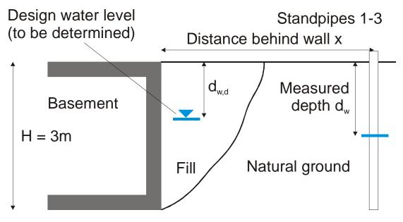
This example is designed to compare engineers' assumptions about water pressures acting on the face of a basement wall. The wall will NOT be provided with a drainage system. Ground surface behind the wall is horizontal will be paved in the long term.
